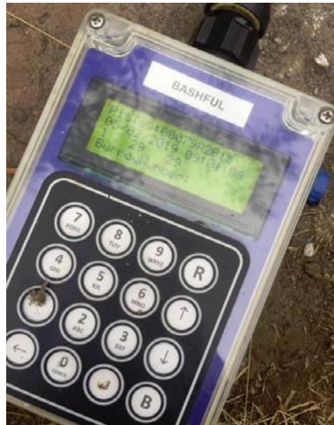
Image 9: The screen of the scanner after a microchip has been detected.
